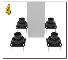
Install the four bases centered on the previous marks using the anchors provided. See our bollard installation instructions if you are unfamiliar with this step.
