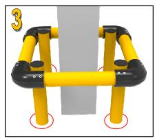
Mark the floor to create the center points for installation of the bases. Inspect for potential interferences such as steel plates and footers. Disassemble the frame to move it aside.
