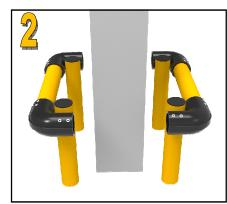
Assemble the horizontal pipes completely into the elbows and loosely tighten one or two set-screws to hold the complete frame in place.
