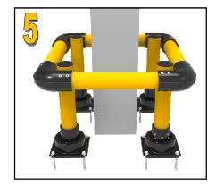
Loosely re-assemble the frame onto the bases. It may be necessary to complete the frame rotated 45° then use wood planks and a fork lift to position the frame into the bases.
